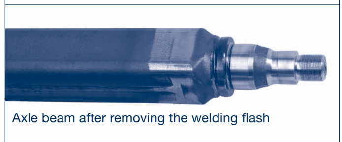
Axle beam after flash butt-welding
